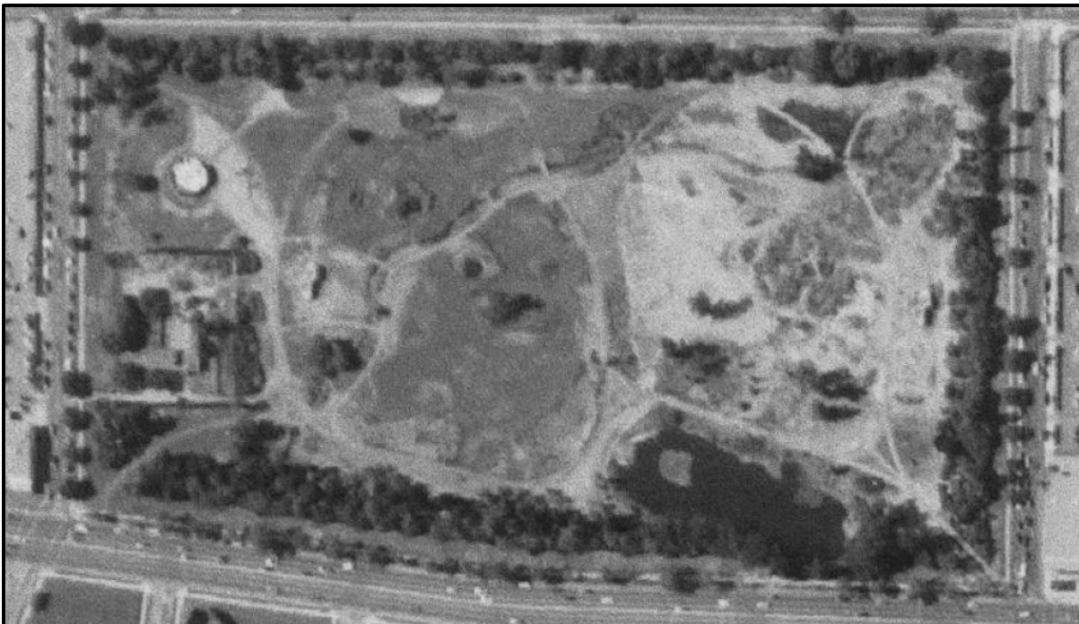
Figure 34. 1952 aerial photograph illustrating the phased execution of the 1948 plan, including the reconfigured circulation paths, the construction of the Observation Pit museum, and ongoing grading and other site improvements
